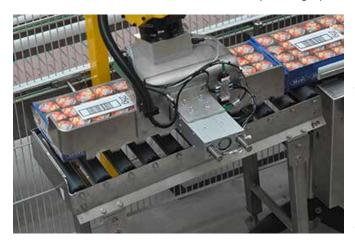
whether the product was filled into jars or aluminium containers. One challenge also involve the behaviour of the foil-wrapped boxes on the gripper shovel. "The jam in the packaging units contained in the boxes is still warm when it arrives at the palletising cell. The temperature is transferred onto the foil and, as result, the box becomes slippery during the gripping
